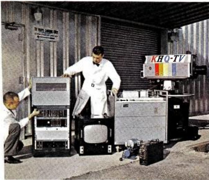
Scene at KHQ-TV loading dock as TK-42 and TR-5 are loaded into panel truck that serves as mobile unit.
